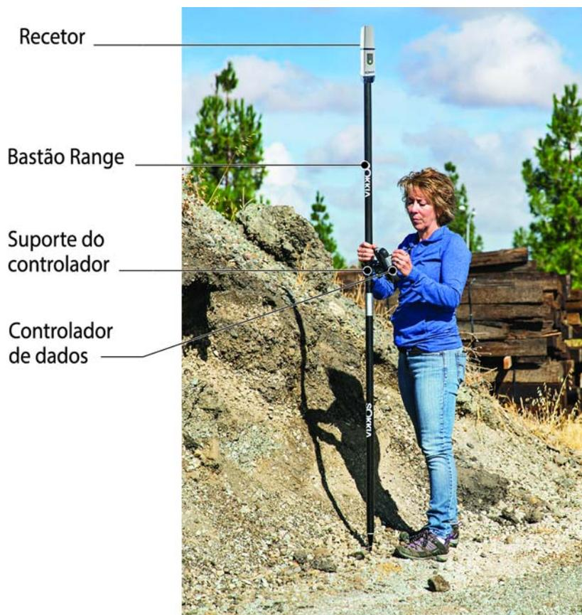
**Figura 23: RTK Rover**
