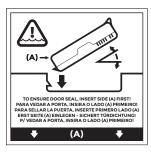
Hold the battery so that the black tab on the front edge of the battery is up and facing the door latch (this tab helps you pull the battery out). Place the back edge in first, gently pushing it underneath the two battery catches. Rotate the front edge down until it is in position.
