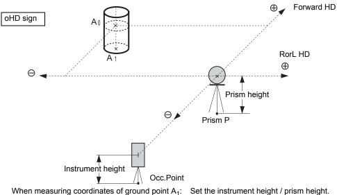
When measuring coordinates of ground point  $A_1$ When measuring coordinates of point  $A_0$ : Set the instrument height / prism height. Set the instrument height only. (Set the prism height to 0 ).
