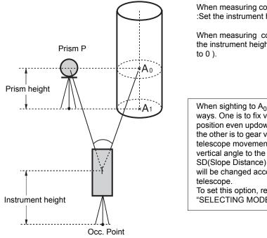
When measuring coordinates of ground point A1 :Set the instrument height/prism height.
