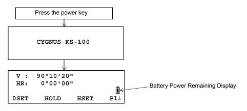
• Confirm the battery power remaining display. Replace with charged battery or charge when battery level is low or indicates "Battery empty". see Section 2.3 "Battery Power Remaining Display".
