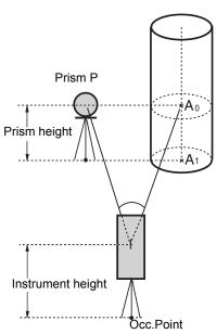
When measuring coordinates of ground point A1 :Set the instrument height / prism height.
