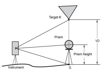
1) With prism height (h) input (Example :h=1.5m)
