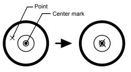
6. Completely Leveling the Instrument
