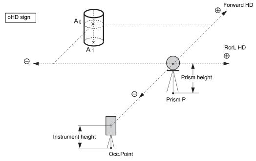
When measuring coordinates of ground point A1: Set the instrument height / prism height.
