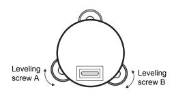
2 Rotate the instrument 90° (100gon) around its vertical axis and turn the remaining leveling screw or C to center the bubble once more.
