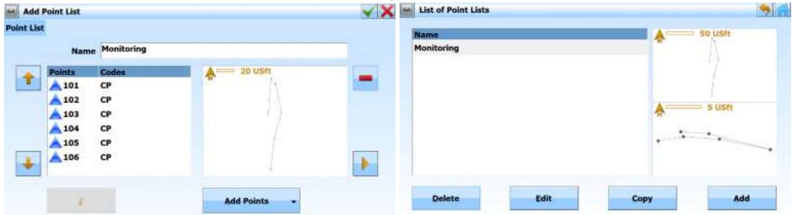
Magnet offers a few horizontal and vertical views of the point list. Sequence of points can also be arranged by using the UP and Down arrows.
