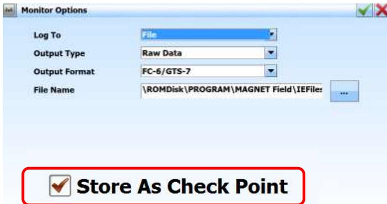
Using this options will allows to easy create a report in Magnet Tools as well to view the points and delta values for XYZ in Magnet field.
