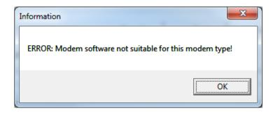
This error message indicates that wrong software version (for example .sff instead of .sf2 or vice versa) has been selected for the hardware of the radio modem.
