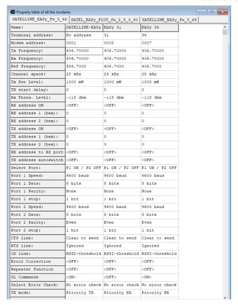
Please note that the settings of the radio modems may also be changed through the property table. The corresponding property table of the radio modem is opened by double clicking the desired column.
