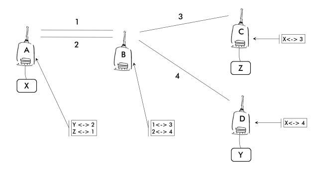
The above figure represents the same network, which has now been configured using the *Virtual Mode Routing*. The difference being that logical links are numbered instead of the radio modems. Operation is easy to understand by thinking of a telephone network realized with traditional overhead wiring.
