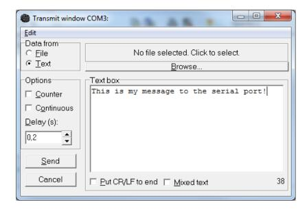
**Continuous** option should be selected if the transmission is to be repeated continuously, in which case the desired delay between packets should be entered into the **Delay** field. The **Counter** option will add a separate serial number to each sent packet.
