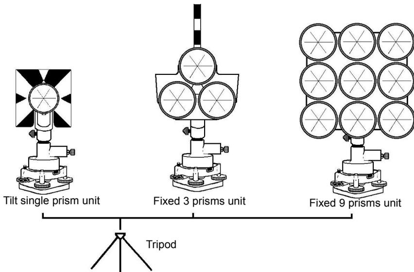
Use the above prisms after setting them at the same height as the instruments. To adjust the height of prism set, change the position of 4 fixing screws.
