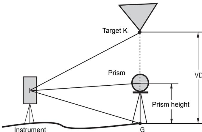
1) With prism height (h) input (Example: h=1.5m)
