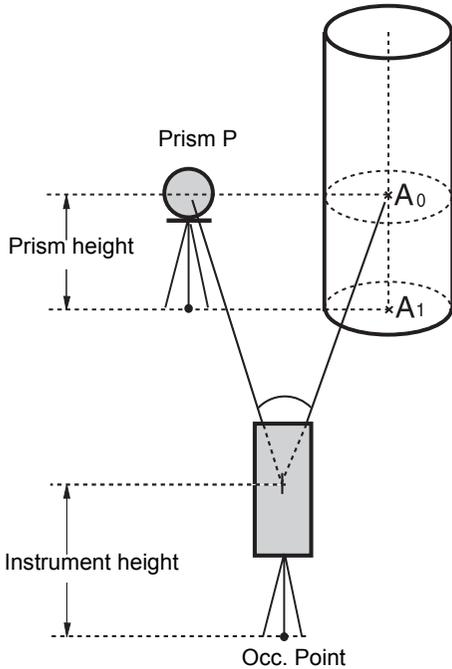
When measuring coordinates of ground point A<sub>1</sub>:
