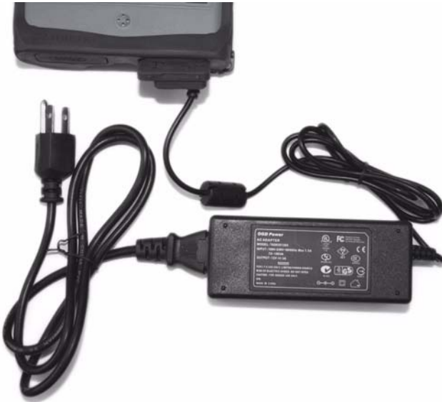
Figure 2-2. Charging the Batteries
