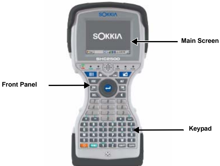
Figure 2-1. Front-Side Components of the SHC2500
