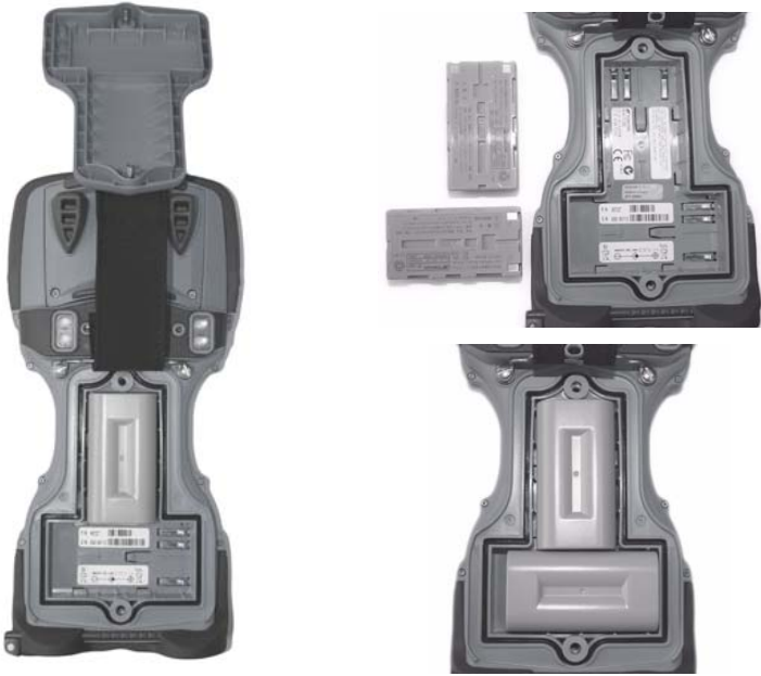
Figure 2-3. Changing the Li-Ion Battery Pack for the SHC2500
